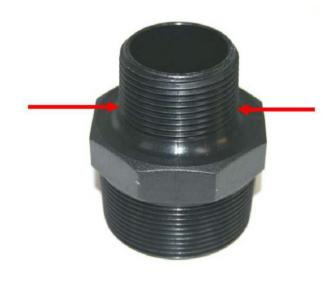
To accurately identify any BSPP or BSPT fitting, measure from one side of the thread to the other and refer to the chart above. EG: If the fitting measured 33.249mm across, it is a 1" BSP fitting and you would refer to it as a 1" BSP fitting. A 2" fitting would measure 59.614mm across the threads, it is called a 2" BSP fitting.
